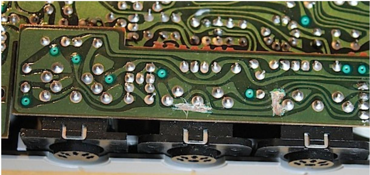
Solder 2 wires, if you want, you can scrape some green mask of the PCB . Don't use leadfree solder here!
