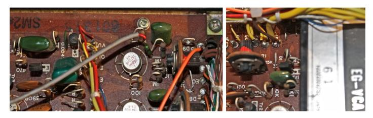
The red wire with the grey shielding is CV2. It goes to a 470k resistor and then to the positive input of opamp 8. CV2 can control volume and the filter using the potentiometers on the back of
