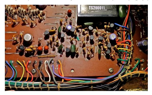
In the following picture you can see the green wire that goes to the collector of the transistor coming from connection 11.
