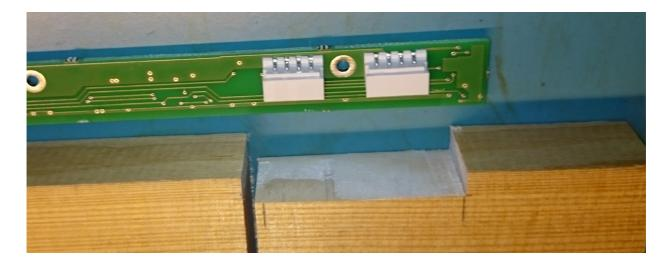
3. Place the board over keys and align all 4 PCBs so the hall sensors (little black thingies) are more or less in the middle of each key. Few milimeters off center is perfectly OK, as long as it's not the edge of a key. Mark PCB locations on the board.
