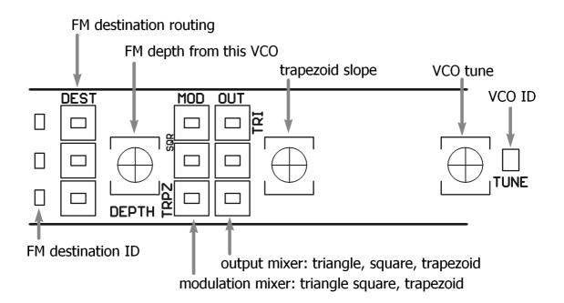
Another controls available are frequency and trapezoid's slope. The slope can be changed with a potentiometer from triangle up to nearly square.
