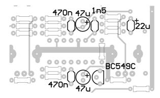
In the next batch you might solder all remaining components at once, that is electrolytic capacitors, film capacitors, transistors and LED. Yes, there's one LED onboard, showing actually only if power is on. That's because no circuit is completed without at least one light source. Better yet if it blinks, but not in this case, as it's connected straight to power line via resistor.
